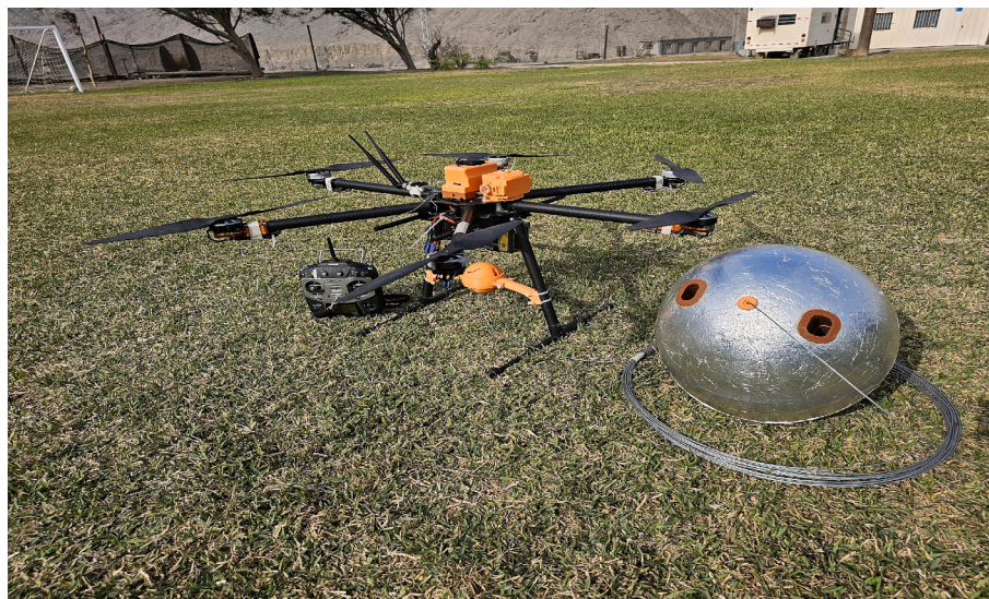
Fig. 3. UAS used for the calibration, alongside the spherical target.
