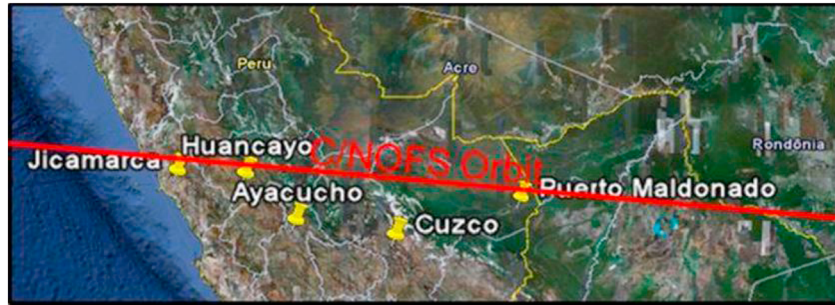
Figure 1. Trajectory of the C/NOFS satellite relative to the five station tomography receiver chain in Peru. The CERTO beacon on C/NOFS transmits 150 and 400 MHz to the ground receivers for measurements of relative total electron content (RTEC) between the satellite and receiver. These TEC data are augmented with in situ electron density measurements on the satellite and ground ionosonde data to yield 2-D images of electron density.
