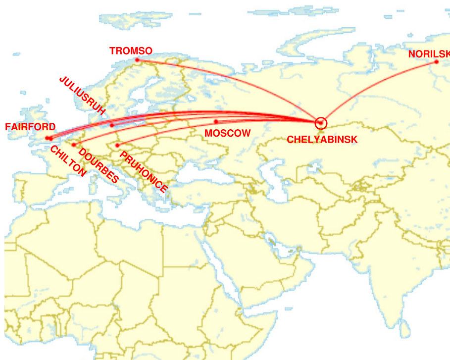
Figure 2. A geographic map of great circle arcs from Chelyabinsk (the meteor explosion site) toward several ionosonde stations located in Europe and Russia, using rectangular projection. The meteor explosion happened on 15 February 2013 at approximately 03:20 UTC.
