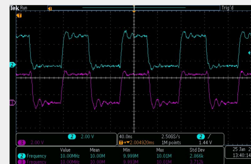
Figure 7. Synchronization between the GPS signal and that generated by the system.
