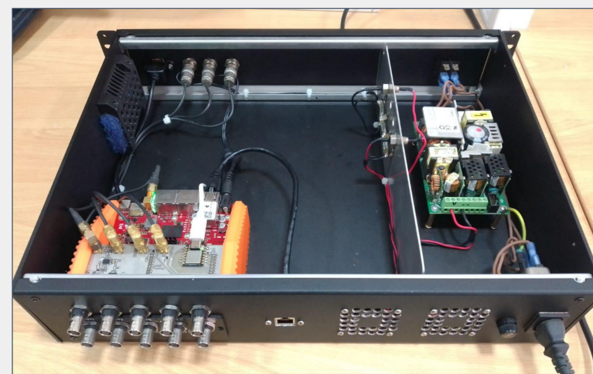
Figure 6. RF Signal Generator Rack.
