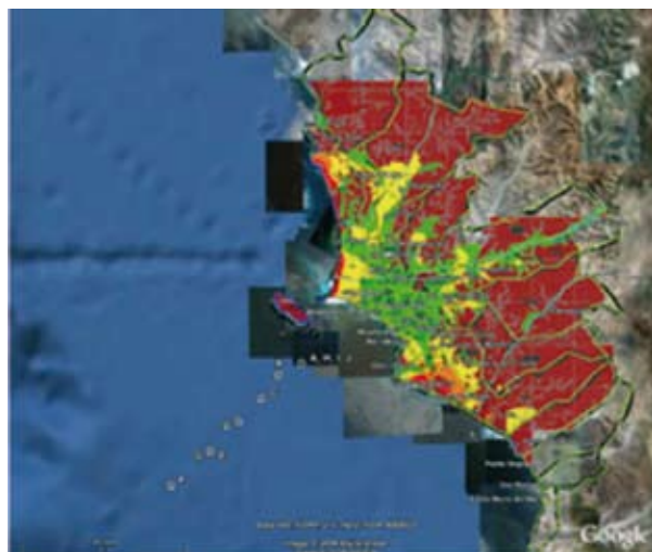
FIGURE 2: Microzonation of Lima metropolitana. The urban area is divided into colored zones corresponding to 4 types of soil; S1 for rock, S2 intermediate soils, S3 flexible soils and S4 for exceptional conditions (map from CISMID, 2004). Yellow line polygons mark the district boundaries (more in Appendix A). The center of energy release (epicenters) for the scenarios A through J are marked by stars.
