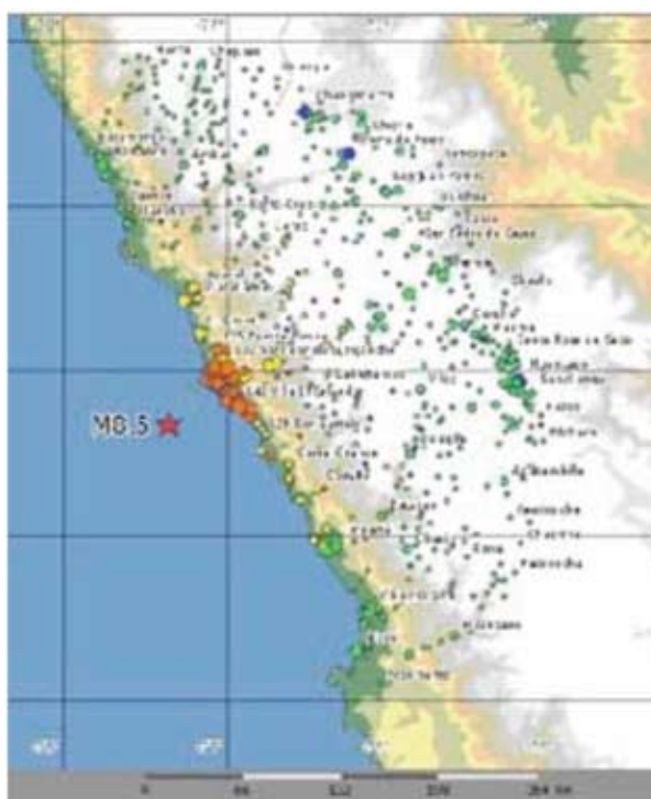
FIGURE 5: Mean damage grade expected in settlements of central Peru in case of an M8.5 earthquake at 30 km depth 40 km offshore Lima. The star marks the epicenter. The sizes of dots are proportional to the population. Orange signifies a damage grade of 3 on a scale of 5, meaning significant damage. Green marks light and blue minor damage, respectively.
