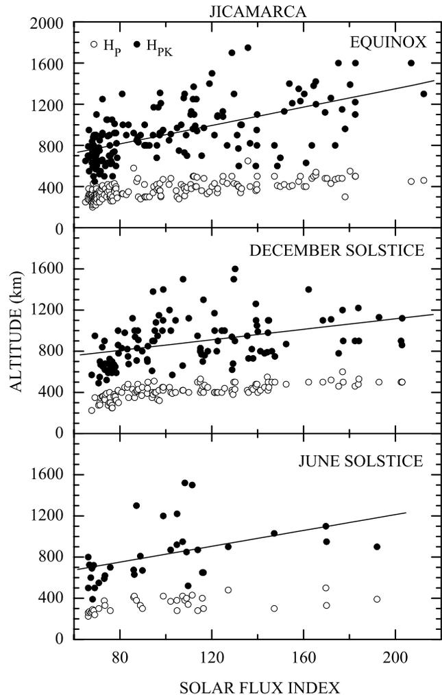
**Figure 6.** Scatterplots of radar plume onset ( $H_P$ ) and peak ( $H_{PK}$ ) heights as a function of solar flux. The straight lines indicate least squares fits to the peak altitude data.
