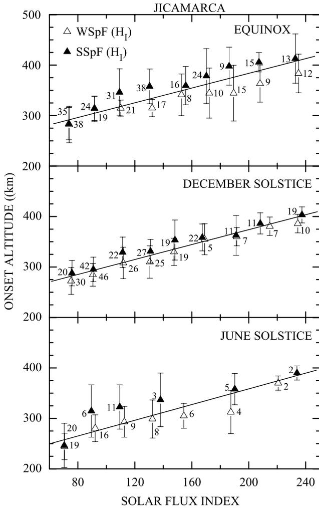
**Figure 3.** Onset altitudes of weak and strong spread  $F$  as a function of solar flux index. The number of samples and standard deviations are also shown. The straight lines denote the least squares fit to the combined weak and strong spread  $F$  data.
