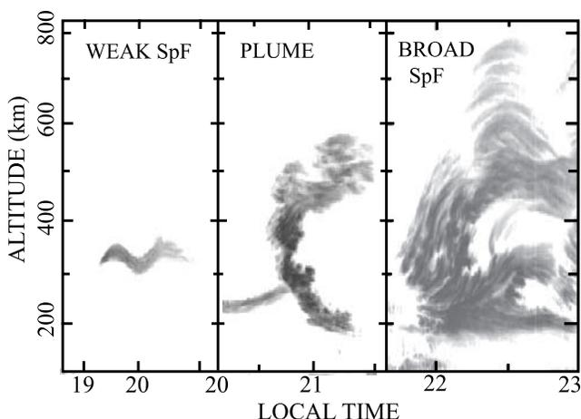
**Figure 1.** Range-time-intensity (RTI) plots of (left) weak spread  $F$  on 3 November 1999, (middle) plume on 9 September 1996, and (right) broad spread  $F$  on 12 September 1996, measured by the JULIA.
