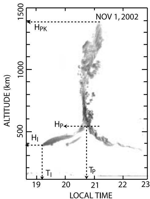
**Figure 2.** Typical JULIA radar plume over Jicamarca on 1 November 2002, illustrating the spread  $F$  parameters considered in this study.  $T_I$  and  $H_I$  correspond to spread  $F$  onset time and height, and  $T_P$ ,  $H_P$ , and  $H_{PK}$  are the plume onset time, height, and peak height, respectively.
