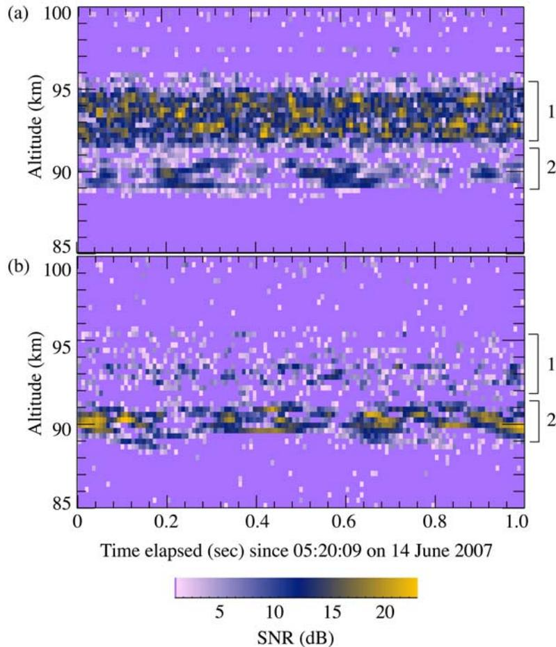
**Figure 3.** High-resolution RTI plot of a part of a trail for the meteor echo shown in Figure 2 at the time indicated by the arrow on the time axis, as observed from the (a) Jicamarca radar and (b) Carapongo radar. The difference in the structure of the upper long duration trail (93–95 km) and the lower-altitude long duration trail (90 km) can be clearly seen in the Jicamarca radar. The lower-altitude long duration is seen to be comprised of small blobs from both the radars.
